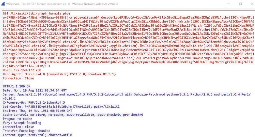
Figure 4-48. The successful exploitation of the tikiwiki vulnerability
